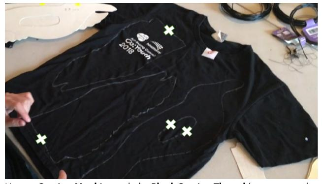
Using a **Sewing Machine** with the **Black Sewing Thread** (using a straight stitch), sew ON the **Chalk** line border of the wing pattern and the body of the bird pattern.
